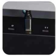
USB cables are connected in the rear locked compartment.
